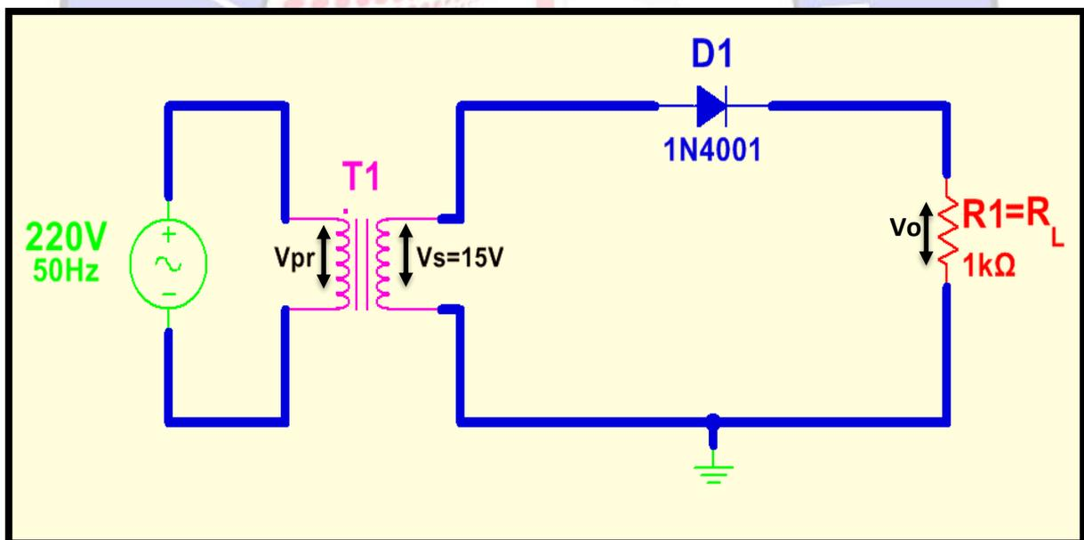
Figure 1: Half-Wave Rectifier with Transformer-Coupled Input Voltage
