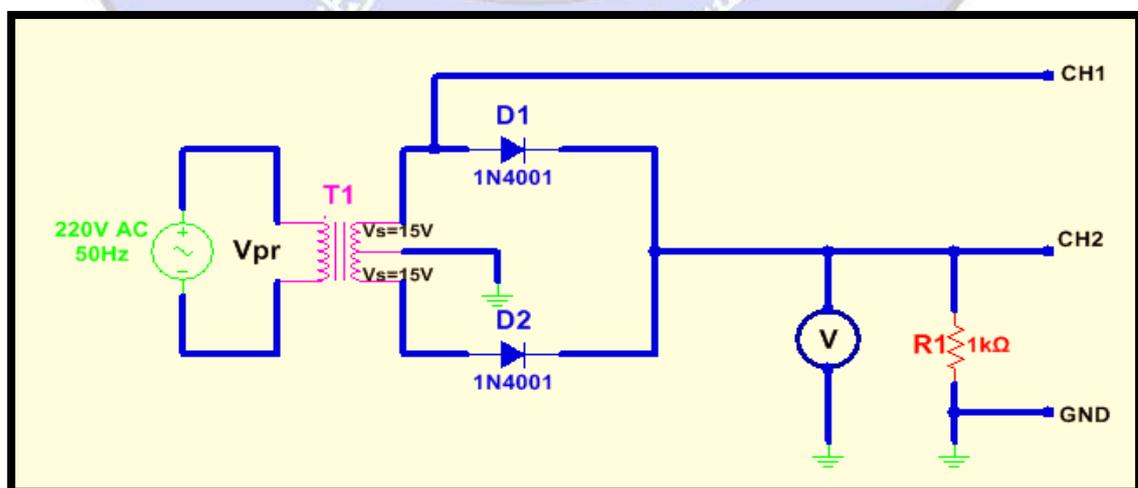
Figure 10: Practical Circuit for the Center-Tapped Full-Wave Rectifier
