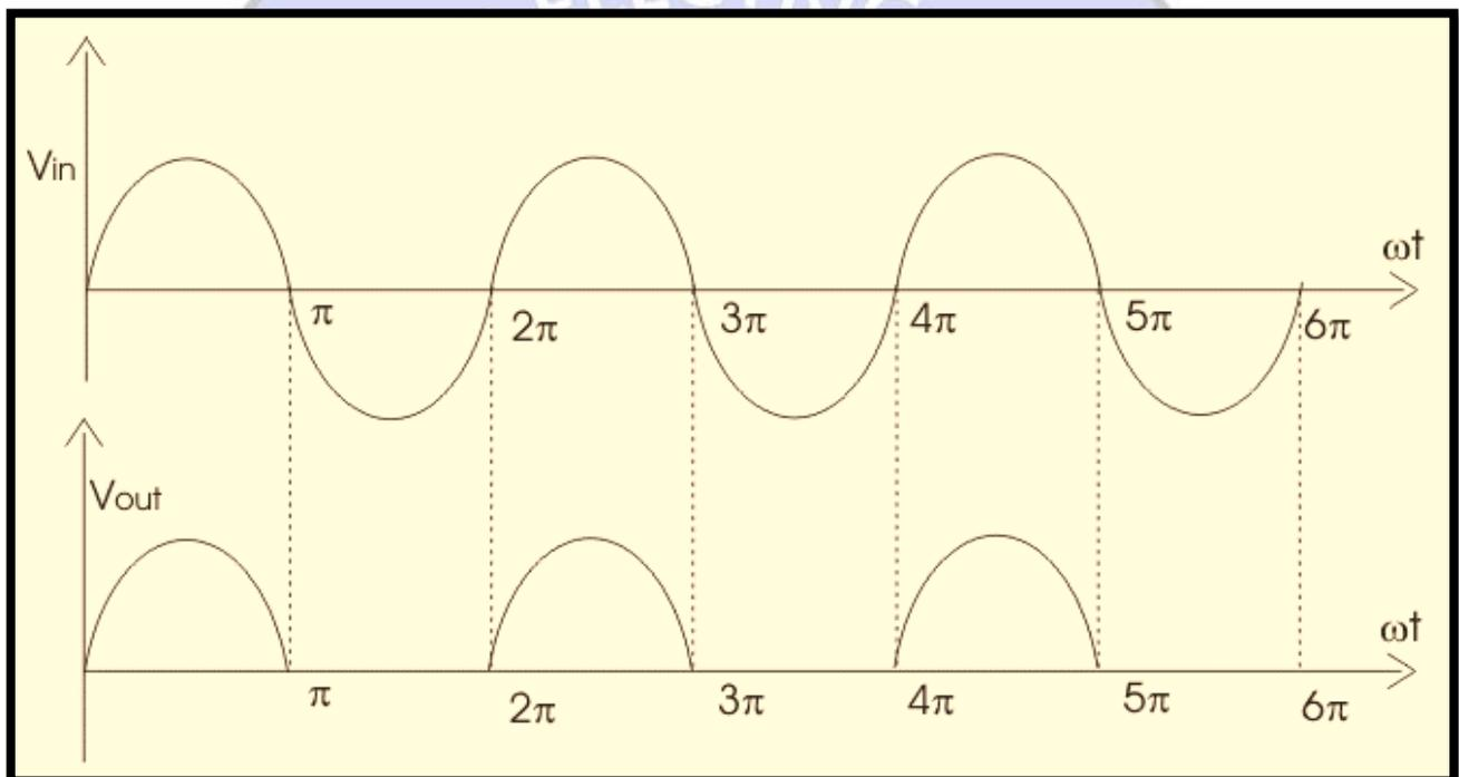
Figure 2: Waveforms of the Half-Wave Rectifier Circuit
