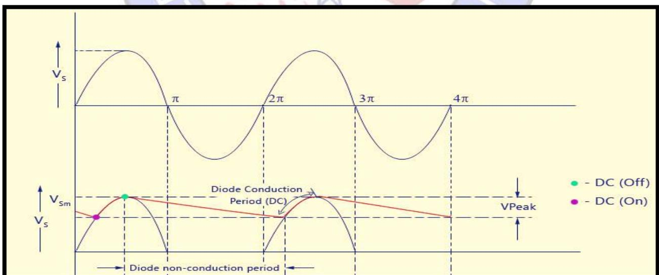
Figure 7: Output Waveform of the Capacitor Filter
