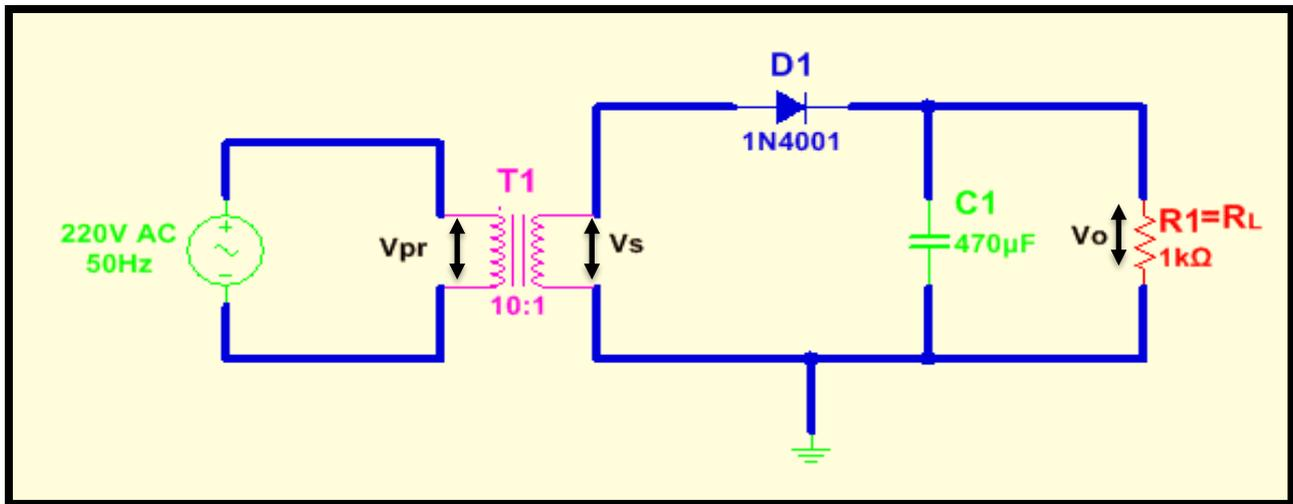
Figure 6: Half-Wave Rectifier with a Capacitor Filter
