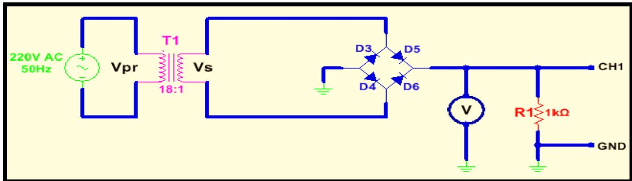
Figure 12: The Practical Full-Wave Bridge Rectifier Circuit
