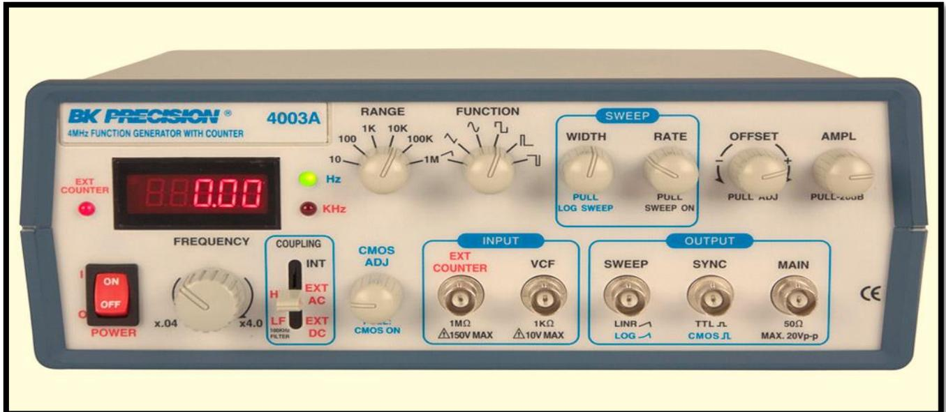
In addition to producing sine waves, function generators may typically produce other repetitive waveforms including sawtooth and triangular waveforms, square waves, and pulses. Another feature included on many function generators is the ability to add a DC offset.
