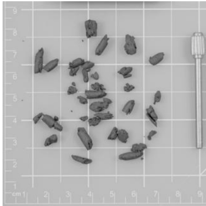
FIG. X2.7 Example of Soil at the Plastic Limit
