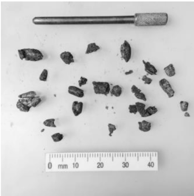
FIG. X2.2 Example of Soil at the Plastic Limit
